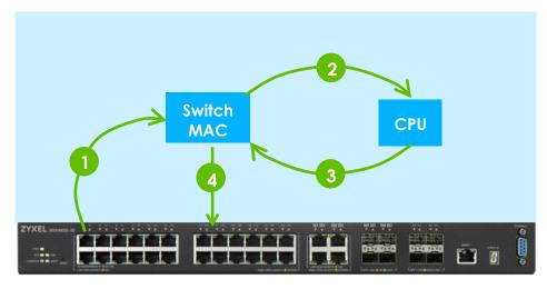
Figure 3: Packet Flow for CPU Forwarding
