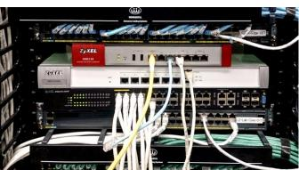
Image 2: Zyxel gateway, WLAN controller, L2 PoE switch were used during the event (from top to down)
